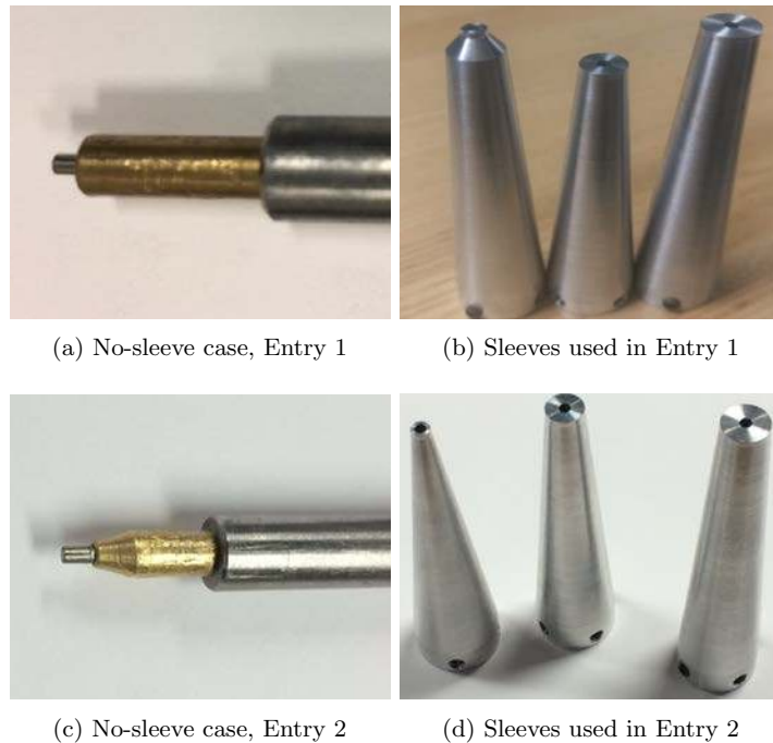
Figure 15. Pictures of pitot probe geometries used in the experiments.
