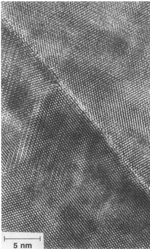
Fig. 8. High-resolution image of a grain boundary devoid of any amorphous phase (Ch12, sample 5).
