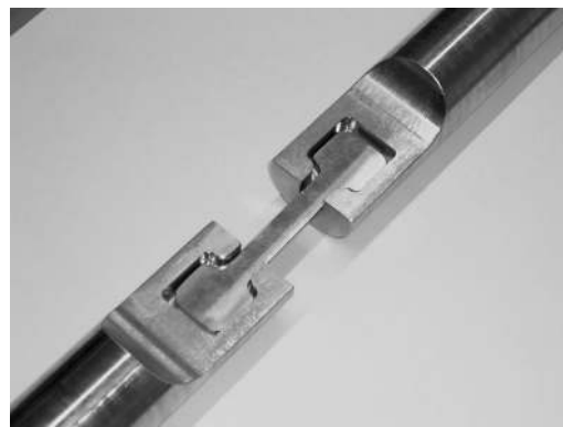
Fig. 1. View of a tensile specimen installed in the fixturing device.
