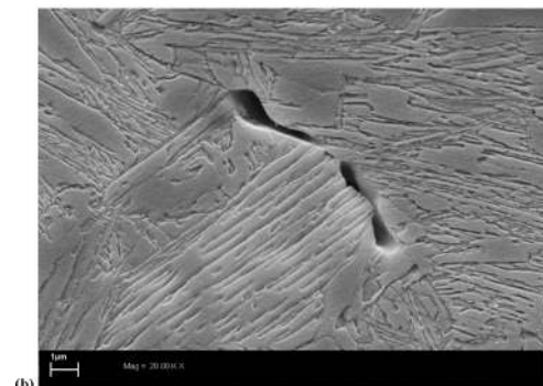
Fig. 5. SEM micrographs of steel B strained by 17% at 950°C.
