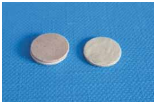
Figure 3. Samples of deposited metallic layers on ceramic pellets for BT_0_S.
