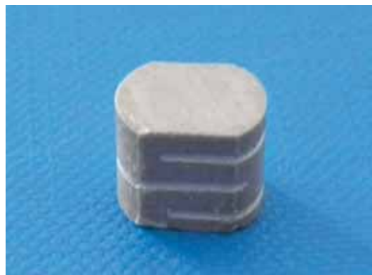
Figure 22. Actuator manufactured from barium titanate ceramic and three metallic layers.
