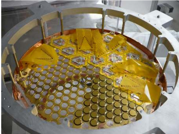
Figure 2: A partially filled LAAPD platter. The triangular platinum-plated contact springs have been installed at the top and right; the LAAPDs at the bottom center have yet not had their contact springs installed.
