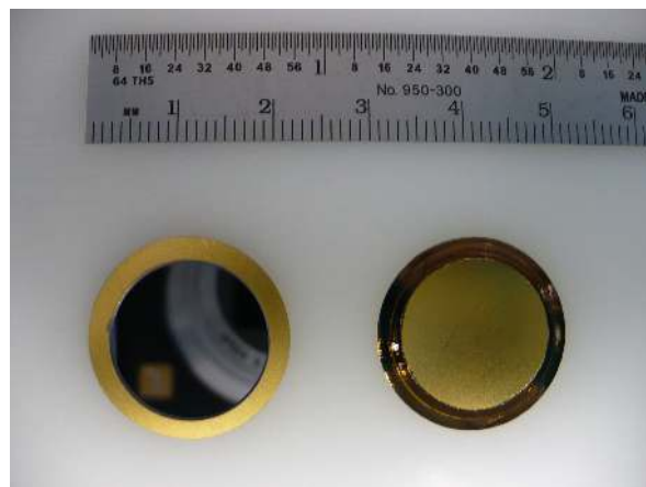
Figure 1: API LAAPD. The ruler indicates the size in cm and inches. The gold-plated cathode is displayed on the right and the active surface surrounded by the gold-plated ring-wafer anode on the left. Note the bevel on the cathode side, providing a longer distance along which to hold the bias high voltage.
