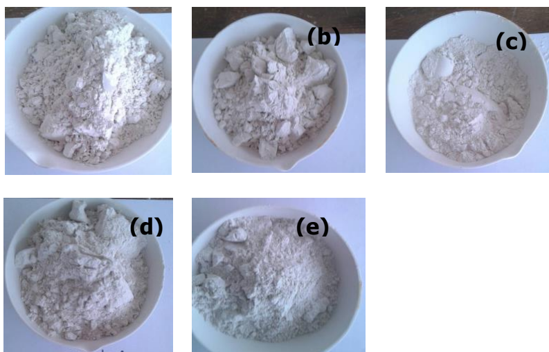
Fig. 1. Optical images of limestone samples at (a) 75 \mu\text{m} , (b) 150 \mu\text{m} , (c) 250 \mu\text{m} , (d) 300, and (e) 425 \mu\text{m} .
