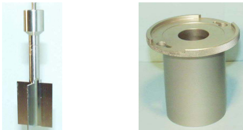
Figure 3-2 Vane rotor (left) and cup (right) used for rheology measurement
