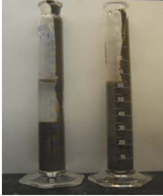
Figure 4-5 Sedimentation of solids from Syncrude MFT after flocculation by Magnofloc 1011 with (left) and without (right) Fe addition after 2 hours
