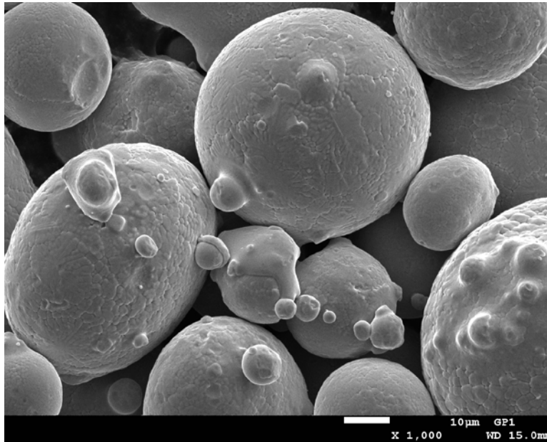
Fig A4. 1000x view of virgin 17-4SS powder. Smaller satellites attached to the particles, a common morphology from powders that are produced via gas-atomization, are evident.
