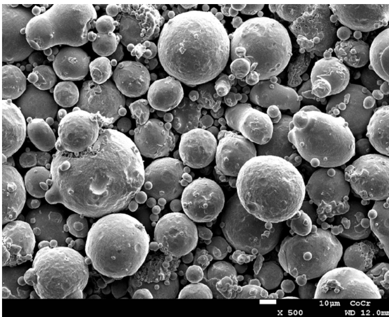
Fig. A15. A 500x view of virgin CoCr powder.
