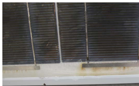
Fig. 2. Region of a module (model 1) after 2000 h in damp heat with + 600 V applied to the active layer with respect to the grounded module frame. There is evidence of grid-finger corrosion and metal-ion transport from the bussing, especially in regions of de-adhesion in the model package seen on the bottom right of the image.
