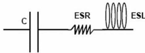
Figure 2.2: Parasitic elements of a capacitor [6]
