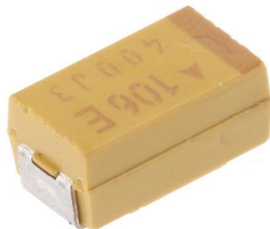
Figure 2.5: Finished surface-mount Tantalum capacitor [14].
