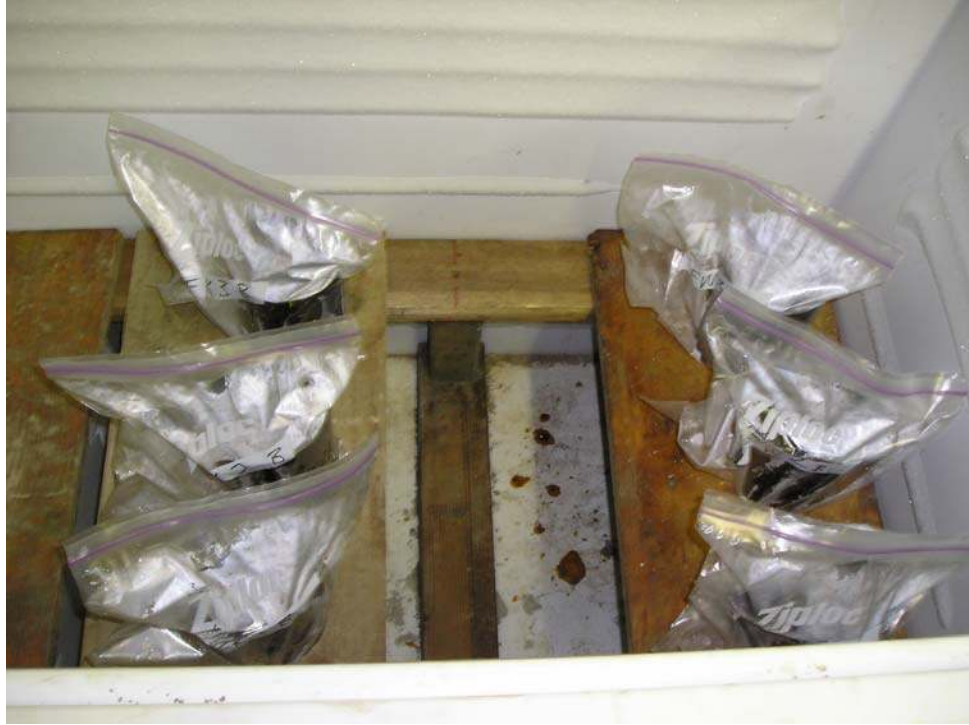
FIGURE 3-7 Freeze-thaw specimens in freezer.
