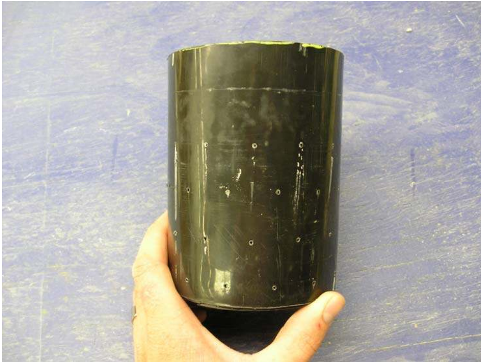
FIGURE 3-6 Specimen mold for stiffness testing during freeze-thaw cycling .
