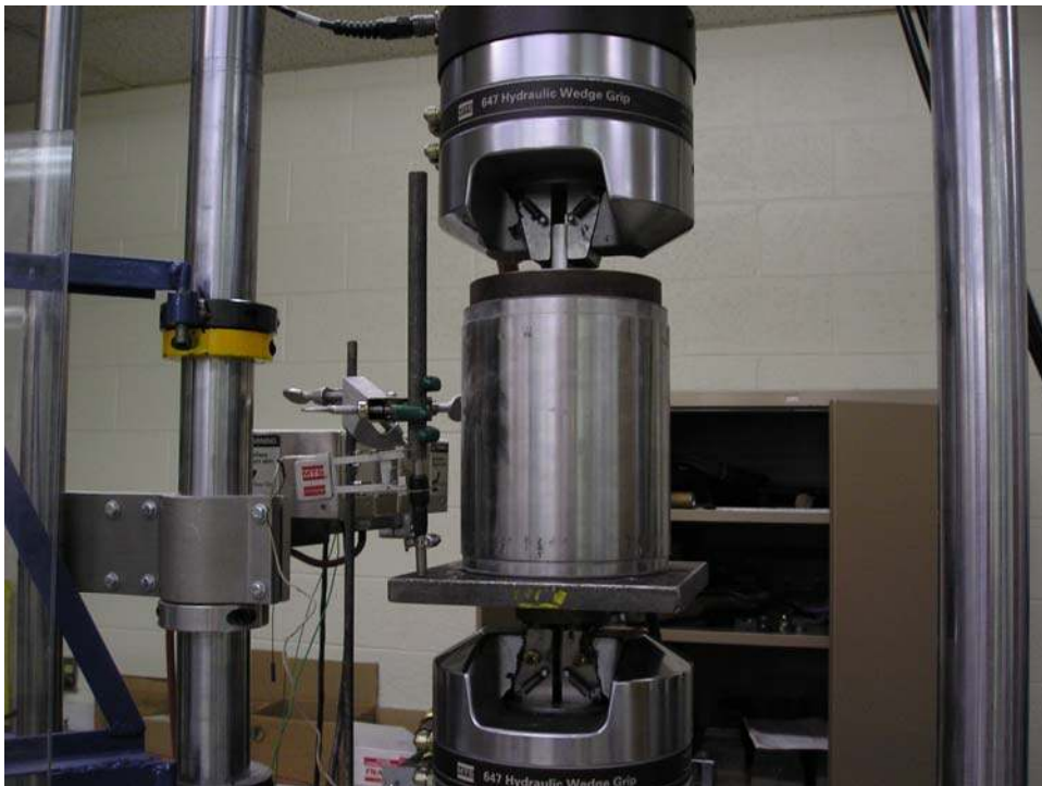
FIGURE 3-1 California bearing ratio testing.
