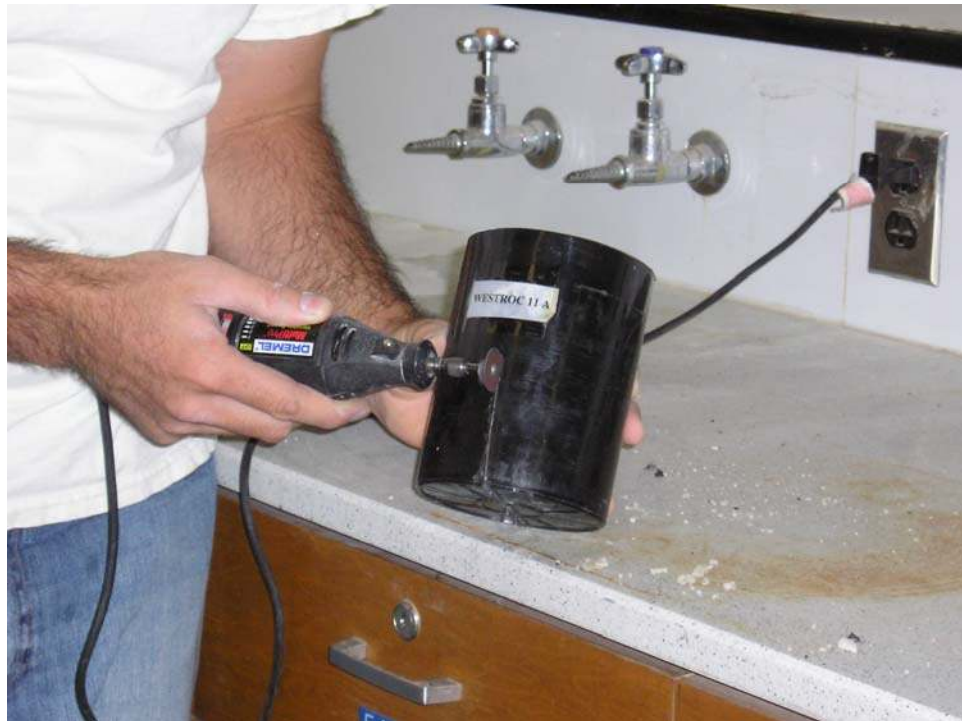
FIGURE 3-2 Removal of plastic mold.
