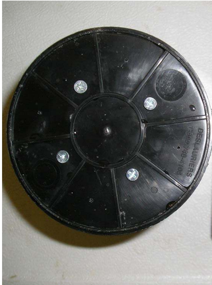
FIGURE 3-4 Specimen mold for stiffness testing.
