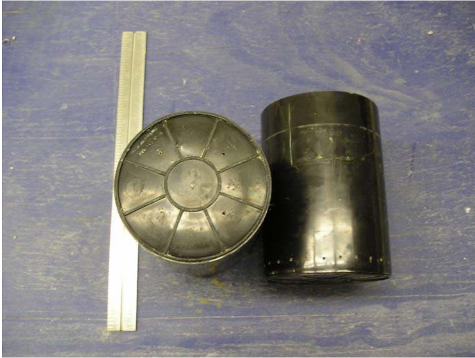
FIGURE 3-8 Specimen mold for tube suction test.
