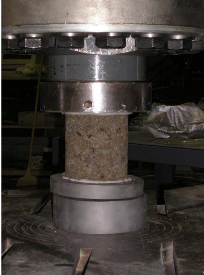
FIGURE 3-3 Unconfined compressive strength test using floating head.
