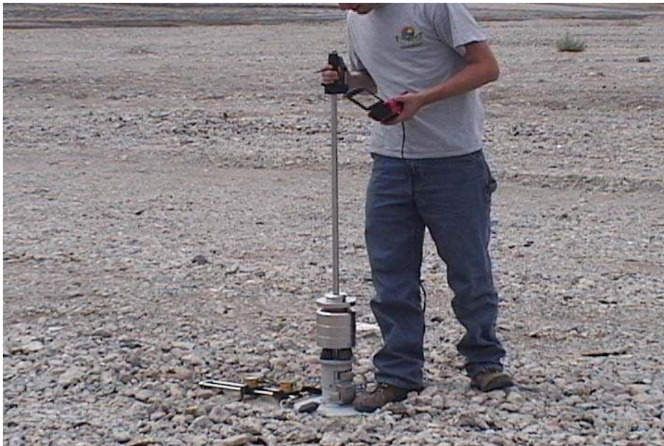
FIGURE 3-13 Portable falling-weight deflectometer.
