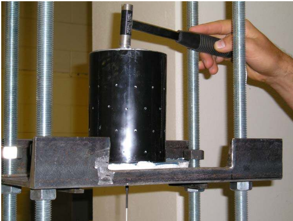
FIGURE 3-5 Specimen stand for stiffness testing.
