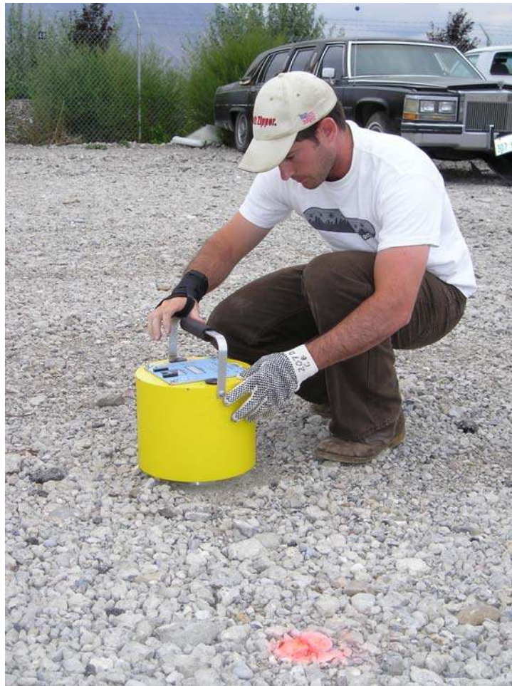
FIGURE 3-12 Soil stiffness gauge.
