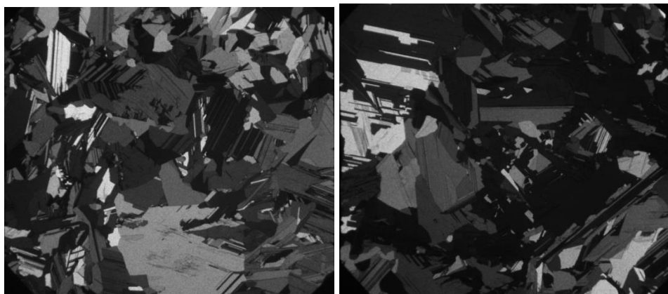
Figure 5-7: NIR transmission images of two multicrystalline wafers used as the XRD verification samples.
