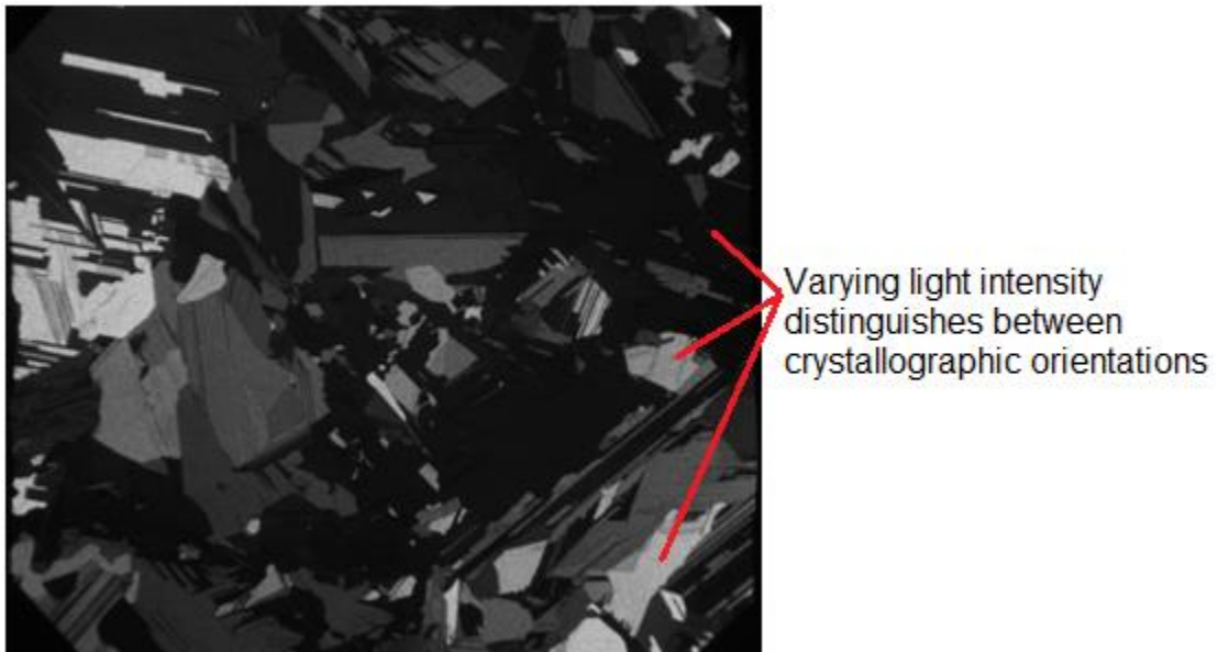
Figure 5-2: NIR transmission image of multicrystalline silicon wafer.
