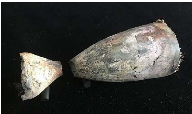
Fig. 11 Deposition of alumina in the nozzle for the propellant 5% aluminum propellants HTPB0514 (after removal from the nozzle contour)
