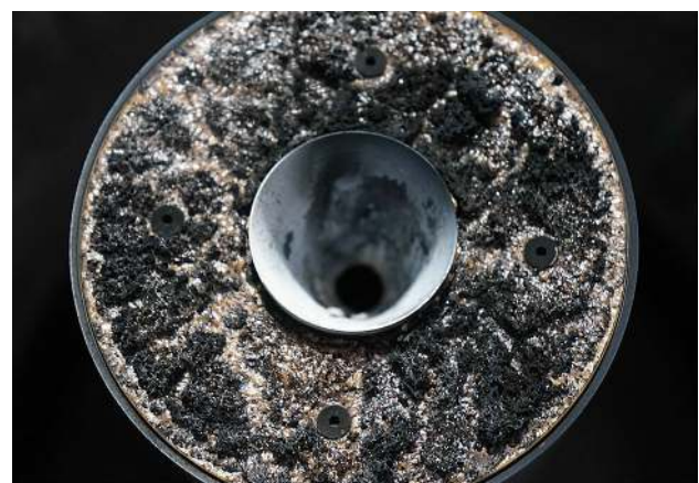
Fig. 8 (Burned) PEEK base plate after a hot firing test
