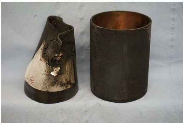
Fig. 6 Thermal insulation of the walls with carbon black insulation coat (left) and a phenolic liner (right) after usage
