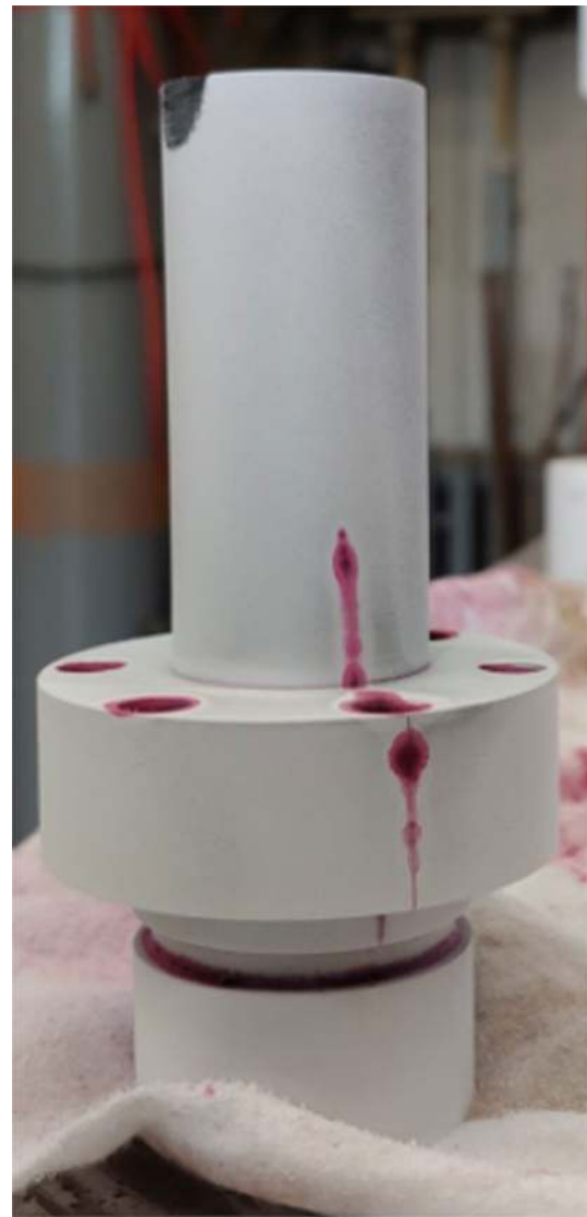
Fig. 7 Penetrant dye inspection of the tungsten nozzle
