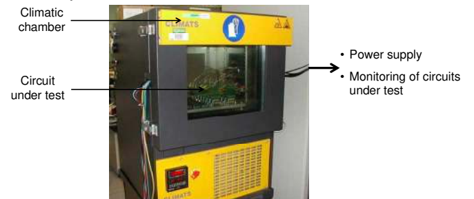
Fig. 9. Climatic chamber for accelerated-life tests
