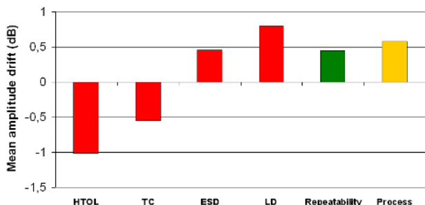
Fig. 15. Emission spectrum mean amplitude drifts after various reliability tests
