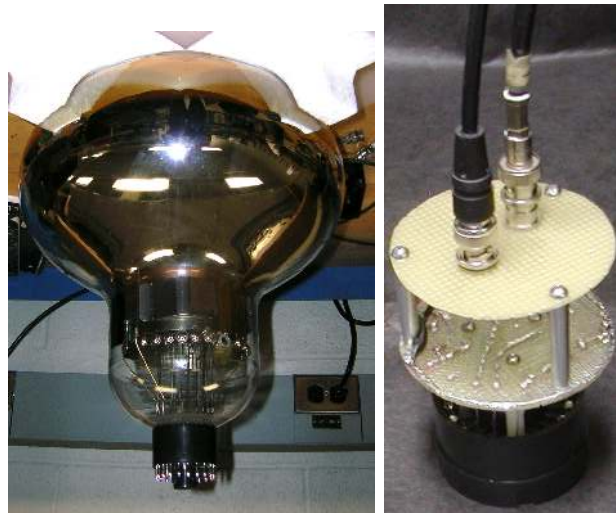
Figure 1: The R11780 12 inch Hamamatsu PMT and the two-cable voltage divider used. The two-cable voltage divider was designed to be cathode-grounded, and the coupling capacitor required to separate the signal from the positive high voltage was included for convenience.
