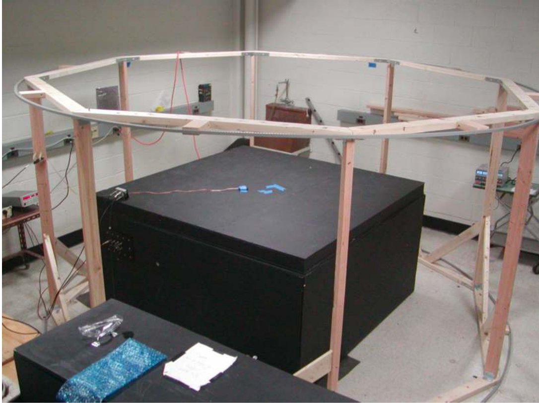
Figure 4: The dark box setup with Helmholtz coils for cancellation of the Earth's magnetic field. At a distance of 1.5 m, the coincidence rate is kept below 5%.
