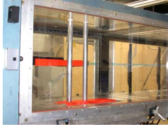
Figure 2. Tandem cylinder configuration in the BART facility.
