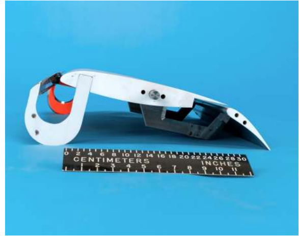
Figure 2: 30P30N airfoil with modified "J" brackets.
