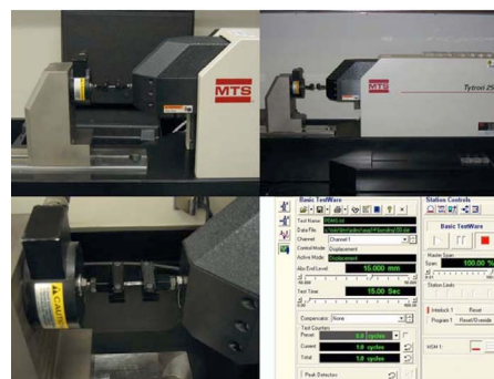
Fig. 1 MTS Tytron 250 microforce tester system (with PDMS samples mounted on two leveled clamps) and control software interface.
