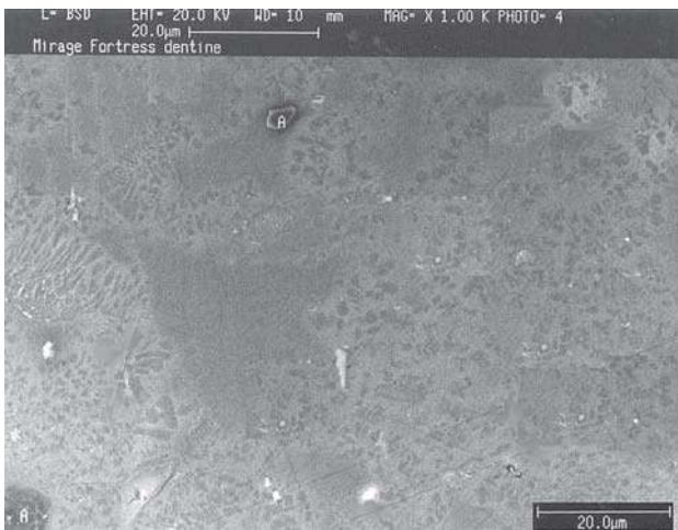
FIGURE 2- Photomicrograph of Fortress (Mirage Dental Systems, Kansas City, KS, USA), a leucite reinforced ceramic. BSI of the microstructure; dark particles (A) are alumina ( Al_2O_3 ). Note that leucite crystals are dispersed in the glass matrix and no cracks are found 17
