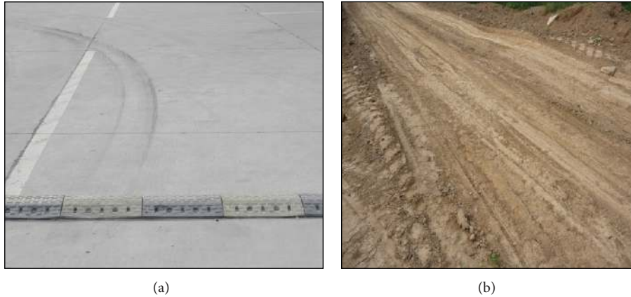
FIGURE 8: Illustration of the test road conditions. (a) Bumped road and (b) unpaved road.
