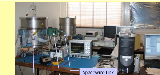
Thermal enclosure containing Caliste 64 and 241 Am source
