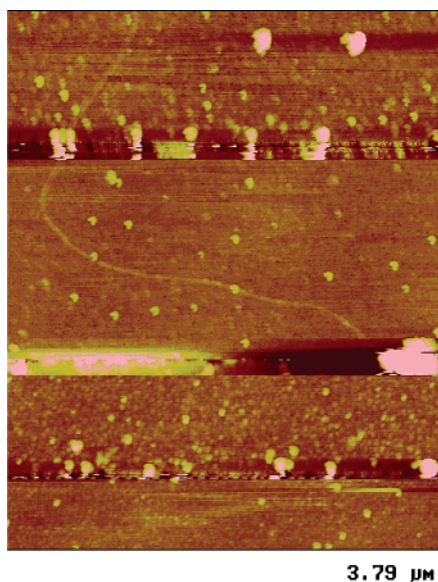
Figure 1. AFM image of a nanotube device after a brief incubation with protein. Individual proteins and clumps of proteins are observed to be adsorbed both to the silicon oxide substrate and to the nanotube.
