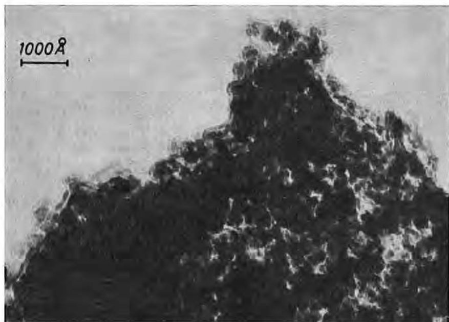
Fig. 5.1. Electron micrograph of particles which are formed in a partially hydrolyzed 1-molar \text{Fe}(\text{NO}_3)_3 solution ( \text{OH}^-/\text{Fe}^{3+} \approx 2 ) after ageing at room temperature for 48 hours. Hydrolysis has been carried out with 4-molar \text{NH}_4\text{OH} .
