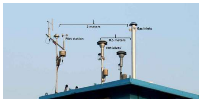
Figure 5. Picture of the co-located instrument inlets and meteorological sensors ( \sim 20 m a.g.l.) at the IISER Mohali atmospheric chemistry facility.
