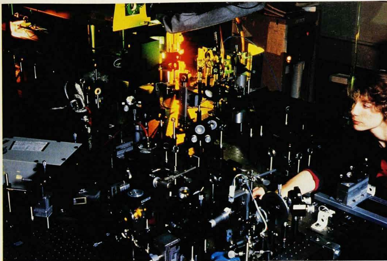
Femtosecond dye laser system at the University of Chicago. Graduate student Sandra Rosenthal makes an adjustment in the copper-vapor-laser dye-amplified system just behind the flowing sample. The system was used to collect the data shown in figure 4. Figure 1
