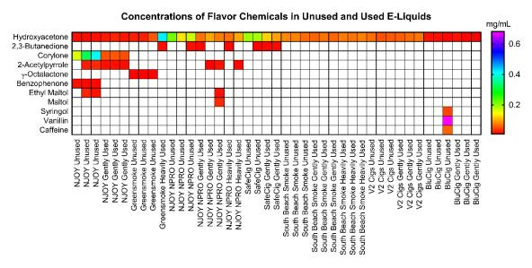
**Figure 3.** Heat map showing the concentration of flavor chemicals in aged unused and used e-liquids. Flavor chemicals are presented on the y axis, and EC products and sample types are on the x axis. All concentrations are in mg/mL White boxes indicate the flavor chemical was not detected.
