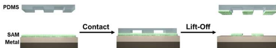
Figure 1. General scheme for chemical lift-off lithography. An oxygen-plasma-activated polydimethylsiloxane (PDMS) stamp is brought into contact with a metal or semiconductor surface functionalized with a self-assembled monolayer (SAM), in this case, 11-mercapto-1-undecanol. Lift-off of the PDMS stamp removes SAM molecules only in the contacted regions, patterning remaining SAMs on the substrate surfaces.
