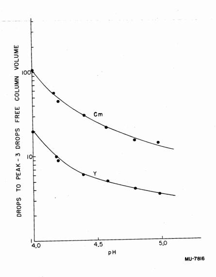
Fig. 5--Elution peak positions versus pH of lactate eluant.
