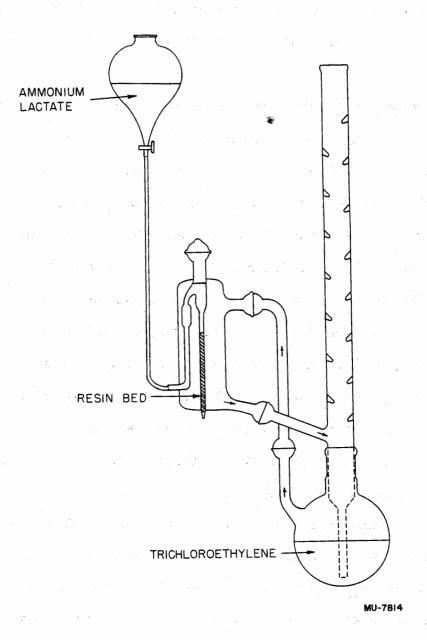
Fig. 3--Column apparatus for separations with lactate.
