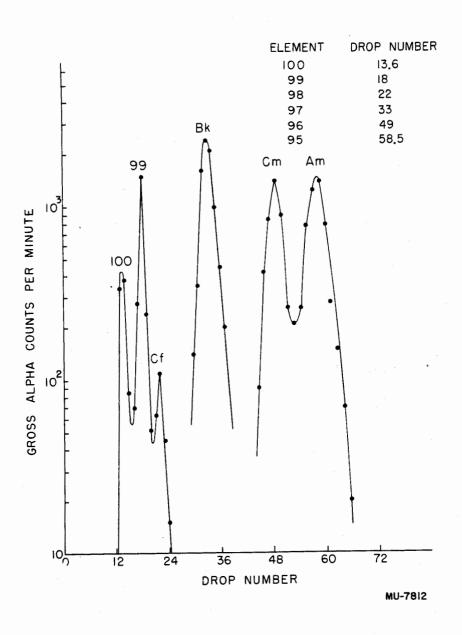
Fig. 2a--Elution of tripositive actinides from Dowex 50 with ammonium lactate eluant ( $\sim$ 2 minutes per drop with 35 $\lambda$  drop size).
