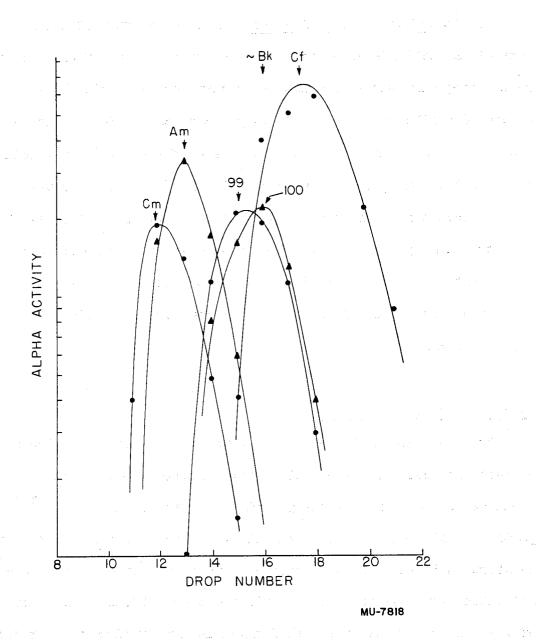
Fig. 7--Elution of actinides from Dowex 1 resin with 1.0 M ammonium thiocyanate.
