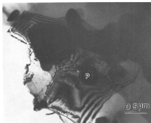
FIG. 21. TEM micrograph showing a representative region of an interface between TiC (marked "T") and reaction products cracked during rolling in a sample heat-treated for 24 h at 913 K. Cracks are normally sharp.
