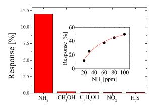
Figure 10: Response of PANI-TiO<sub>2</sub> sensor film to NH<sub>3</sub> (concentration 20 ppm), CH<sub>3</sub>OH (concentration 100 ppm),  $C_2H_5OH$  (concentration 100 ppm), NO<sub>2</sub> (concentration 100 ppm), H<sub>2</sub>S (concentration 100 ppm). The inset shows the response of the sensor to NH<sub>3</sub> as a function of concentration in the range 20-100 ppm. Redrawn and adapted with permission from Ref. [57]
