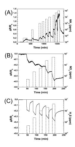
Figure 16: Resistance change  $\Delta R/R_0$  (solid line) and analyte gas concentration (dashed line) as a function of time upon the exposure of different gases. (A): NH<sub>3</sub>; (B): NO<sub>2</sub>; (C): H<sub>2</sub>S. Redrawn and adapted with permission from Ref. [70]
