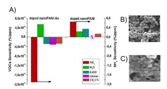
Figure 15: A): Sensitivity of nanoPANI-Au and nanoPANI for ammonia, ethanol, toluene and acetonitrile. B): SEM image of nanoPANI-Au composite obtained from osmosis-based method. (nanoparticles with diameters in the range from 180 to 220 nm). C): SEM image of nanoPANI. Redrawn and adapted with permission from Ref. [69]
