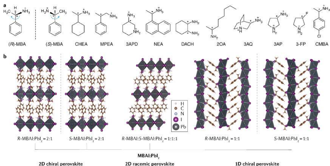
Fig. 4 | Representative chiral ligands and chiral hybrid organic–inorganic perovskites. a | The chiral ligands discussed in this Review: MBA (methylbenzylammonium), CHEA (1-cyclohexylethylammonium), MPEA ( \beta -methylphenethylammonium), 3APD (3-aminopiperidine), NEA (1-(1-naphthyl)ethylammonium), DACH (1,2-diaminocyclohexane), 2OA (2-octylamine), 3AQ (3-ammonioquinuclidinium), 3AP (3-ammoniopyrrolidinium), 3-FP (3-fluoropyrrolidinium) and CMBA (1-(4-chlorophenyl)ethylammonium). Based on the Cahn–Ingold–Prelog (CIP) priority rules, the four groups around a chiral center are prioritized according to the atomic number and priority. This begins with the four atoms closest to the chiral center and moves to subsequent atoms in the event of a tie. With the fourth (the lowest priority) group facing away from the viewer, a path can be traced from groups 1-2-3. If this path is clockwise, the chiral center is designated as R (from the Latin word rectus ); conversely, if it is counter clockwise, the chiral center is designated as S (from the Latin word sinister ). Here, using ( R )-MBA and ( S )-MBA enantiomers as an example, the clockwise and anti-clockwise directions are shown (blue arrow) according to the priority of the four groups. b | Single-crystal structures of
