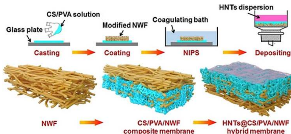
Fig. 7 Schematic depiction for the fabrication process of the HNTs@CS/PVA/NWF hybrid membranes [56]
