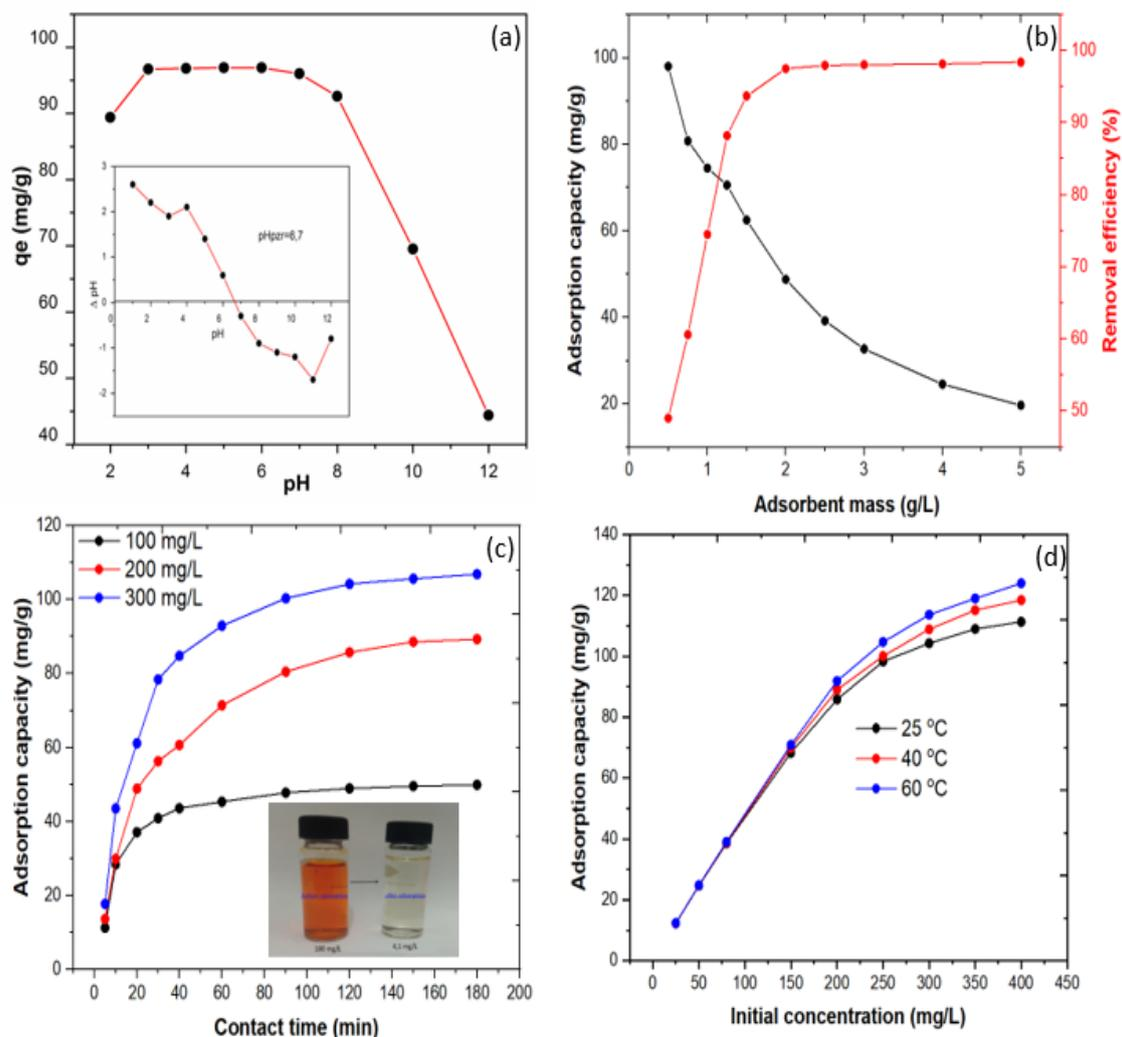
**Figure 3.** Effect of pH (inset: zero point charge plot) (a), adsorbent dose (b), contact time (c), and initial MO concentration (d) on MO adsorption onto CHt@MgO biocomposite.
