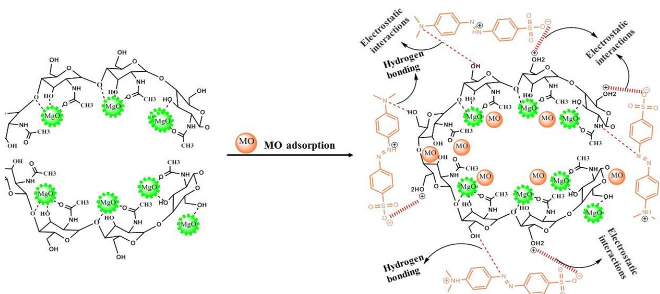
Figure 5. MO adsorption mechanism on CHt@MgO.
