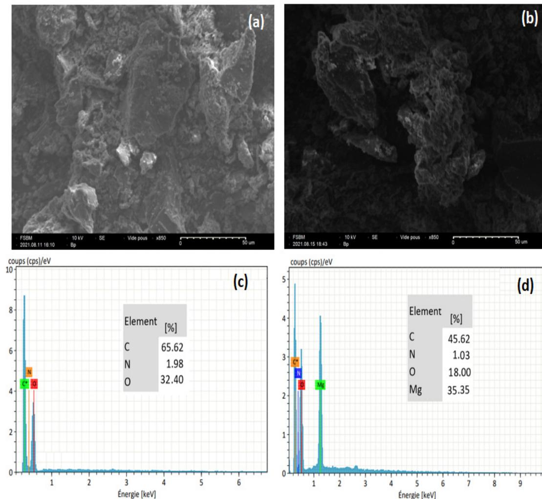
**Figure 2.** SEM images of CHt (a) and CHt@MgO (b); elemental analysis plots of CHt (c) and CHt@MgO (d).
