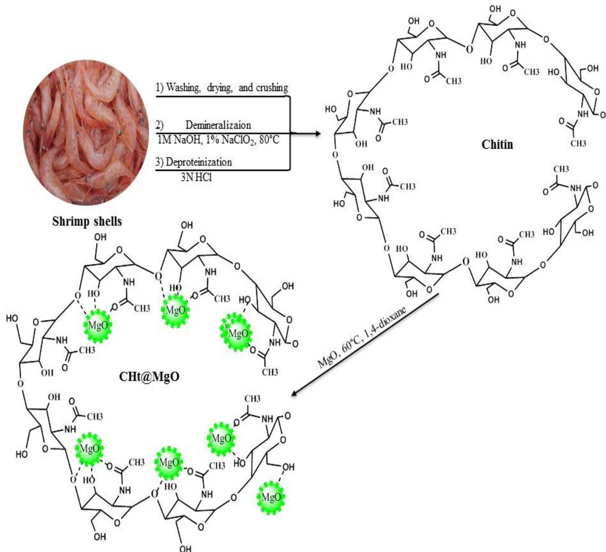
**Scheme 2.** Schematic representation of CHt@MgO biocomposite synthesis.
