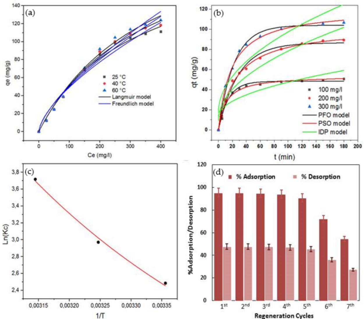
**Figure 4.** Nonlinear adsorption equilibrium isotherm models (a), and adsorption kinetic models (b) for MO adsorption on CHt@MgO; Van't Hoff plot (c) and CHt@MgO regeneration plot (d).
