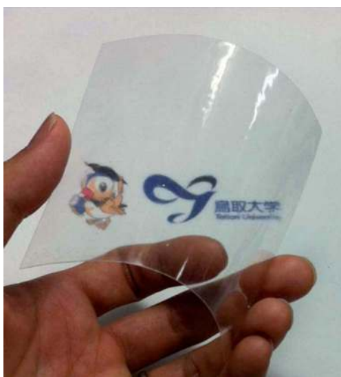
Fig. 14 Appearance of DCP films reinforced with chitin nanofibers. Reproduced from ref. 59. Copyright 2011, the Royal Society of Chemistry.
