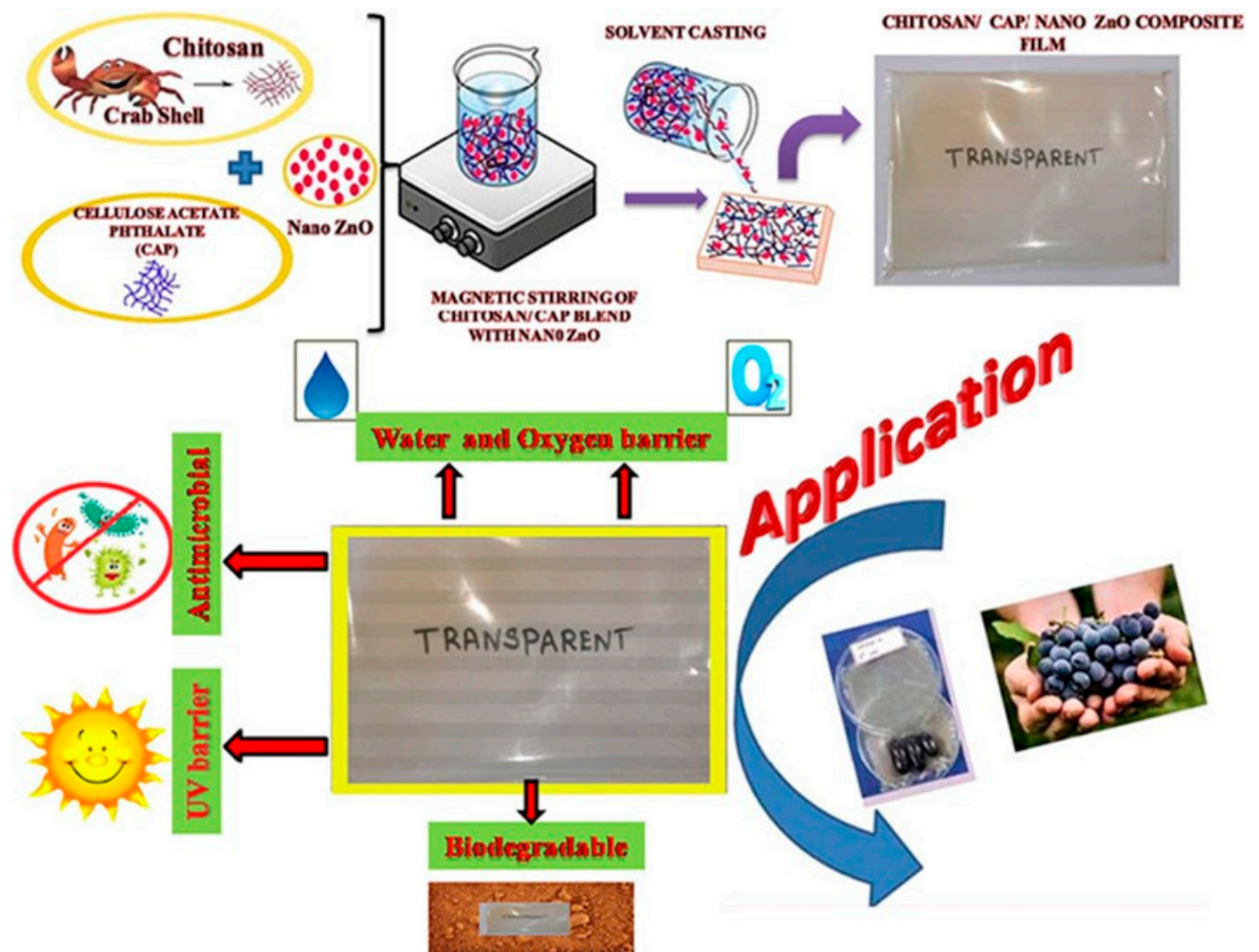
Figure 7. Schematic diagram of CS/CAP and ZnO nanoparticle film preparation and applications [91].
