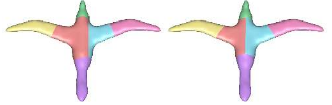
Figure 12: Taking into account the dominant reflective symmetry of a model discourages off-center cuts (left) and results in a more pleasing partition (right).
