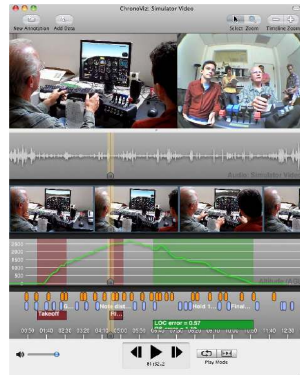
Figure 3: Data from a flight simulation. The data, from top to bottom, show: two videos, a waveform of the audio, individual video frames, a graph of the altitude of the simulated flight with overlaid annotations, several categories of annotations.
