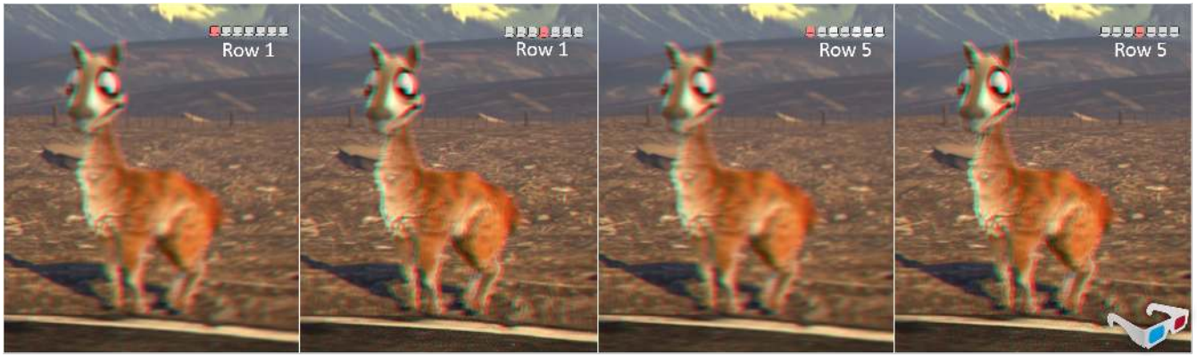
Figure 8: Simulating stereo images from our display, comparing the central vs. leftmost seat in two rows. Images from the extreme seats are somewhat blurrier as discussed in Sec. 3.4. Throughout this paper, the glasses icon denotes content that should be viewed with anaglyph glasses.
