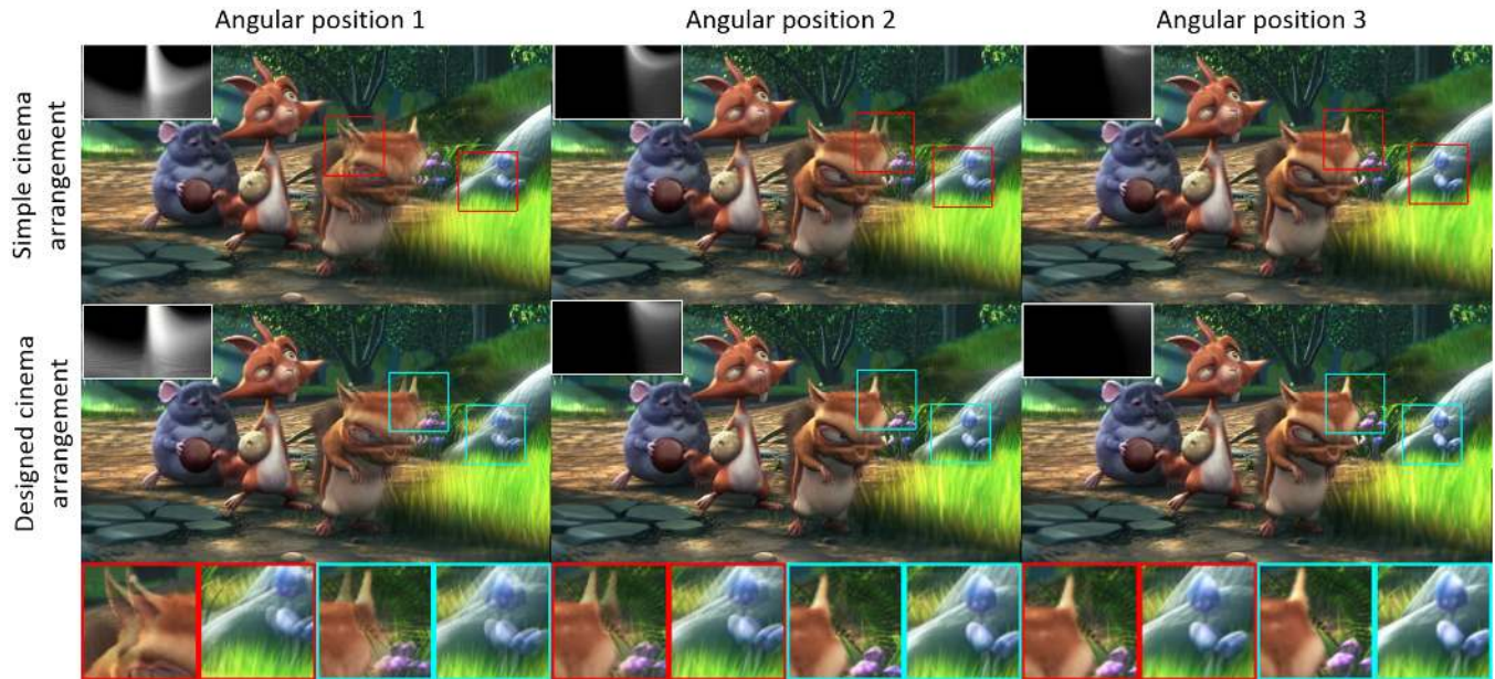
Figure 13: Images perceived at the three leftmost angular positions of the central seat in the first row, for two different cinema configurations. In both cases the extreme angular positions involve more ghosting than the central ones, but when the cinema arrangement is properly designed (2nd row), one can reduce ghosting aberrations in the center of the viewing zone. For better visualization, the bottom row compares enlarged windows from both configurations. The transition map of each viewing position is presented at the top-left corner.
