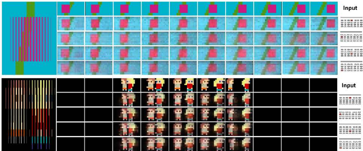
Figure 14: Two test scenes captured through our prototype. The top one illustrates 10 angular shifts of a square floating in front of a flat background, and the second one a few rotated views of pixelated figures. Top row: target angular images. Rows 2-5: angular images captured from different seats, illustrating accurate reproduction of the target. Enlarged animated illustration of the captured images can be seen in the supplementary file. Left: The interlaced angular images as displayed on the back screen. Right: the tested seat marked on the auditorium layout.
