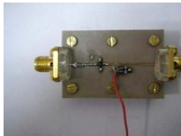
Figure 13. Practical circuit for generating UWB pulse.
