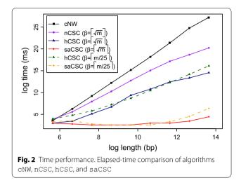
notice that q does not affect the time efficiency of the algorithms. The results in Fig. 2 show that hCSC and saCSC are still the fastest, even though  $m = \mathcal{O}(\beta)$ , and that saCSC is clearly the fastest of all. As expected for  $m = \mathcal{O}(\beta)$ , we observe that hCSC and saCSC become gradually slower as m grows.
