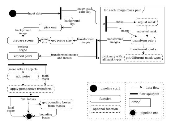
Figure 3. Transformation pipeline activity diagram.
