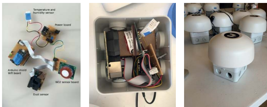
Figure 3.2 Hardware modules of a sensor device (left), and the integration in the casing: open (middle) and closed (right).
