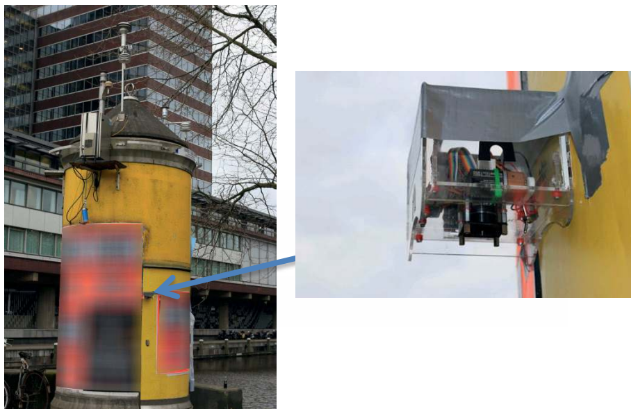
Figure 2.8. An informal measurement point is close to an official station (Amsterdam-Stadhouderskade) for data comparison.
