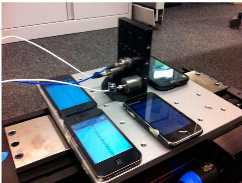
Figure 1. Sinusoidal wave shaking table test setup.
