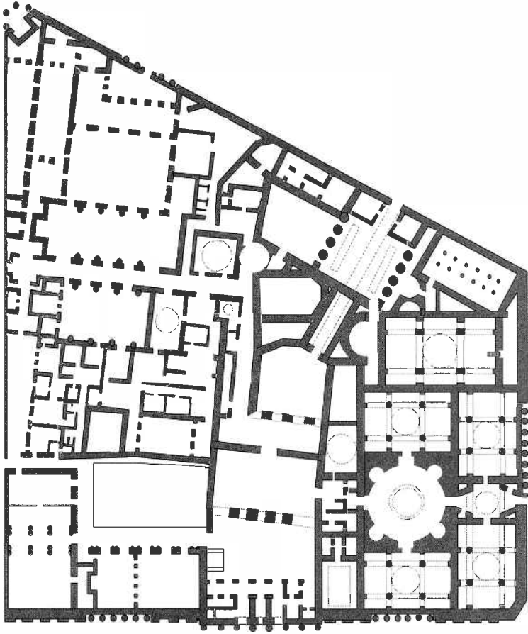
Bank of England, London, by John Soane (1788–1834). Each type of transaction has its own grand hall, and the various activities are connected through an intricate pedestrian circulation system.
