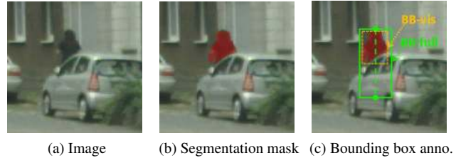
Figure 2: Illustration of bounding box annotations for pedestrians. For each person, the top of the head and middle of the feet is drawn by the annotator. An aligned bounding box is automatically generated using the fixed aspect ratio (0.41). The bounding box covering the segmentation mask is used to estimate the visible part.
