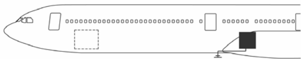
Fig. 2. Position of the CARIBIC container and the inlet system on the Airbus 340–600.
