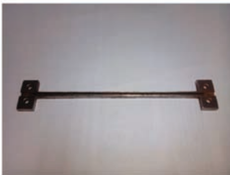
Figure 3: (a) 3D design (b) photograph of fabricated FBG packaging fixture.
