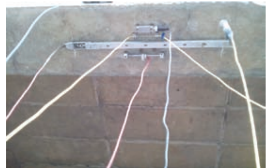
Figure 14: Photograph of the close view of the mounted FBG and other conventional sensors.
