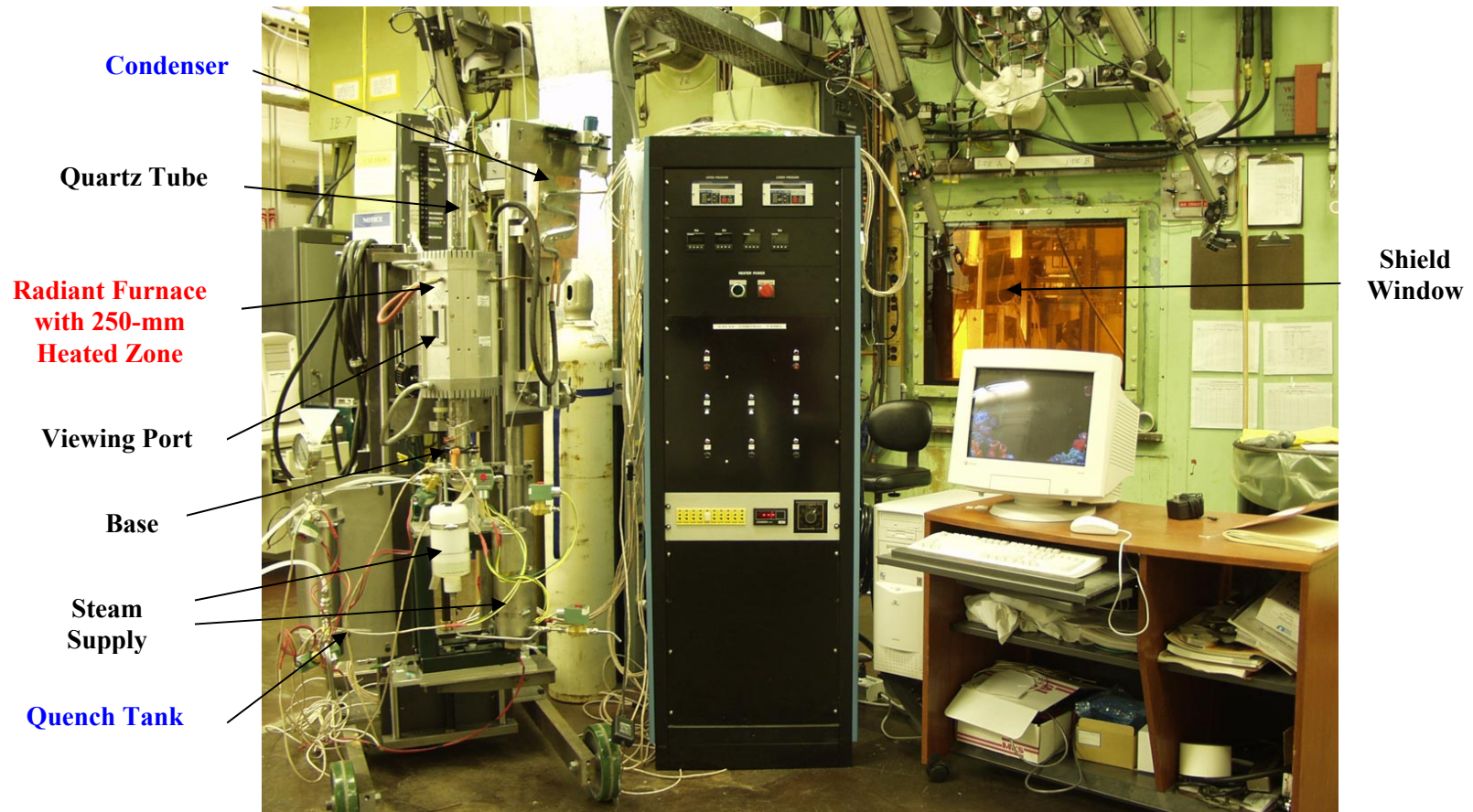
Figure 6. Overview of the out-of-cell LOCA integral test apparatus. One in-cell unit was located at Workstation 6 of the Alpha-Gamma Hot Cell Facility (AGHCF) behind the hot-cell shield and seal windows. High-burnup Zry-4 oxidation/quench tests, as well as high-burnup Zry-2 oxidation and integral tests, were conducted in the AGHCF. Following closure of the AGHCF to programmatic work (January 2006), the out-cell apparatus was moved to a "cold" laboratory for testing nonirradiated cladding samples. This apparatus, equipped with a new furnace and a shorter (610 mm) test chamber, was moved in 2008 into Hot Cell #4 of the Irradiated Materials Laboratory for performing oxidation-and-quench tests with high-burnup ZIRLO and M5 cladding samples.
