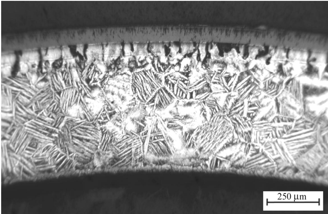
Figure 231. High-burnup Limerick oxidation sample following one-sided oxidation in steam at 1200^\circ\text{C} for a 300-s hold time.
