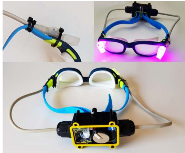
Figure 4: Final version of the prototype: the control button (right), the device working on the ACF mode (right) and a detail of the hardware (bottom).
