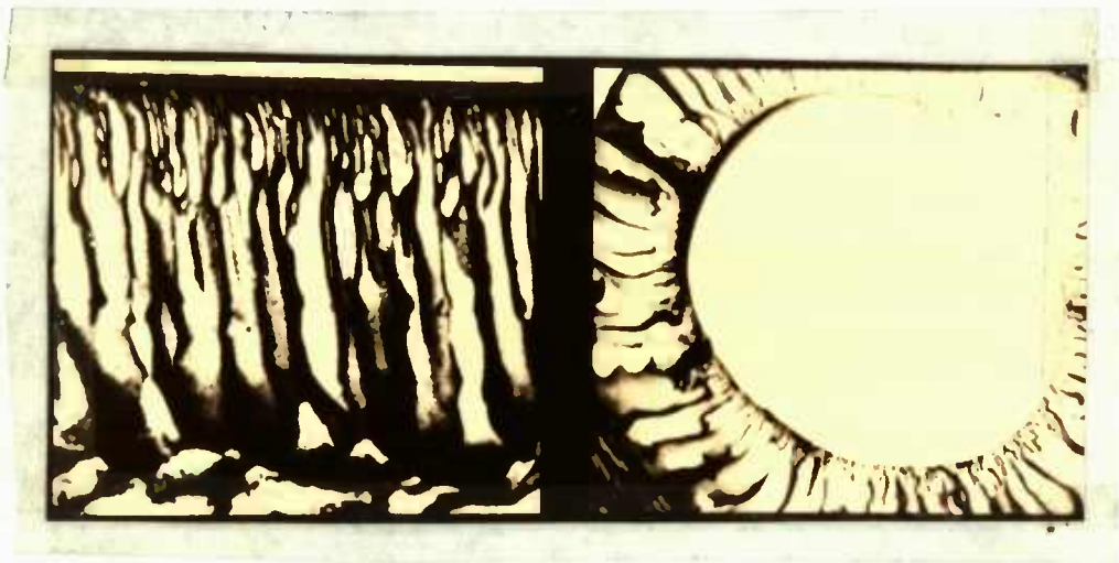
Figure C. Scanning electron photomicrograph (400x) of conventional flat sheet membrane (left) and hollow fiber of similar porosity (right).
